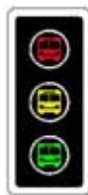
Steady Red Bus Stop bus behind line and wait for green light before proceeding
