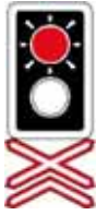
Red Flashing Signal Stop before signal and don't proceed until safe to do so.
