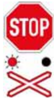
Railway Crossing Red Flashing Signal Train approaching, stop and proceed only when lights stop flashing and it is safe to do so
