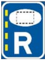
Authorised Passenger Transport Vehicle Lane Right Reservation Sign
