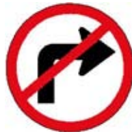
Right Turn Ahead Prohibited
