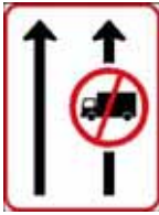
Lane Use Control by Regulatory Sign
